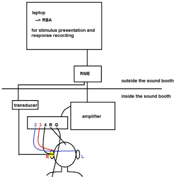
Figure 8. A summary of stimulus presentation and response recording steps in the AEP measurements, shown separately for inside and outside the sound booth.
