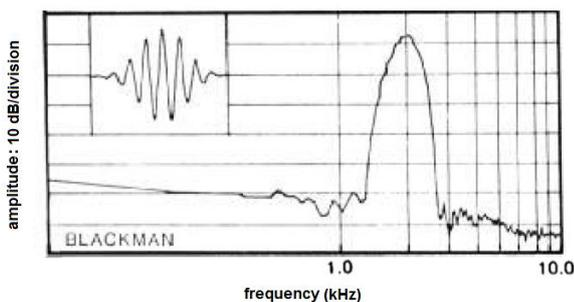
Figure 6. *The time waveform and the amplitude-frequency spectrum for a 2 kHz toneburst having 2 ms rise- and fall times and no plateau. Adopted from Gorga & Thornton (1988).*
