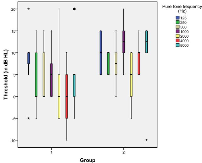
Figure 13. Pure tone thresholds per frequency for subjects in the low noise exposure group (group 1) and subjects in the high noise exposure group (group 2).
