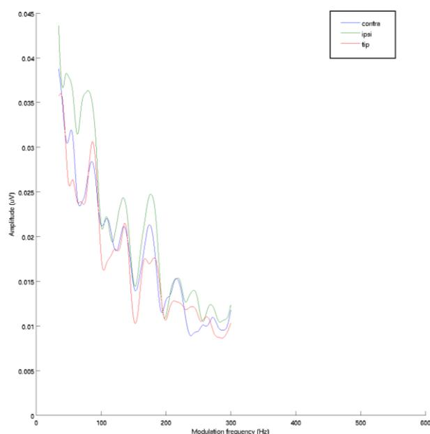
Figure 33. *Grand average ASSR spectrum in response to the noise sweep.*
