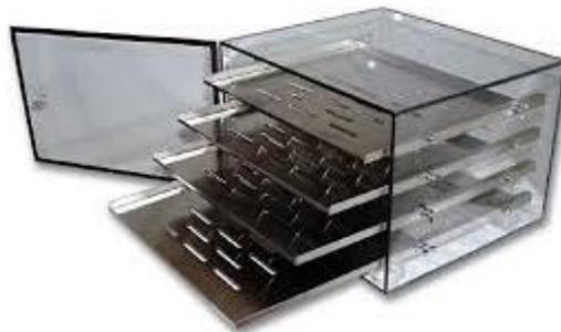
**Figure 13: The Biospherix 'C-chamber sub chamber'.** This chamber was used to create a hypoxic environment (1,7 mg/L oxygen saturation level) in the ADaM.
