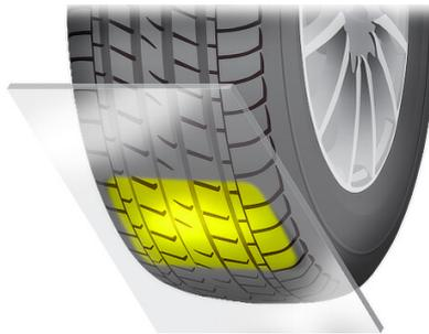
Figure 4.20: Contact patch tyre, [45]
