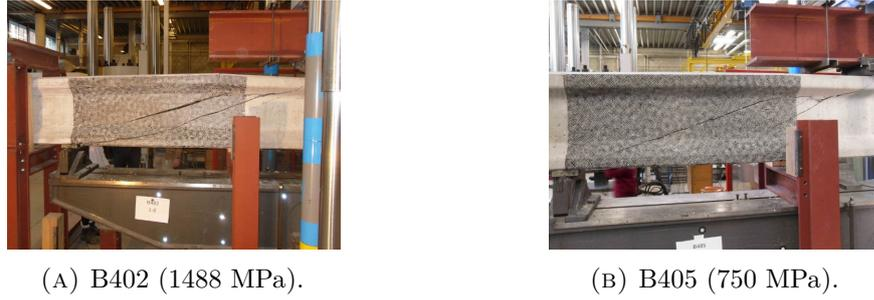
FIGURE 4.5: The amount of prestressing influences the inclination of the cracks and the ductility of the failure.
