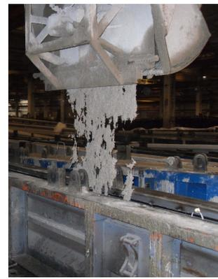
(B) Casting the formwork with SFRC.
