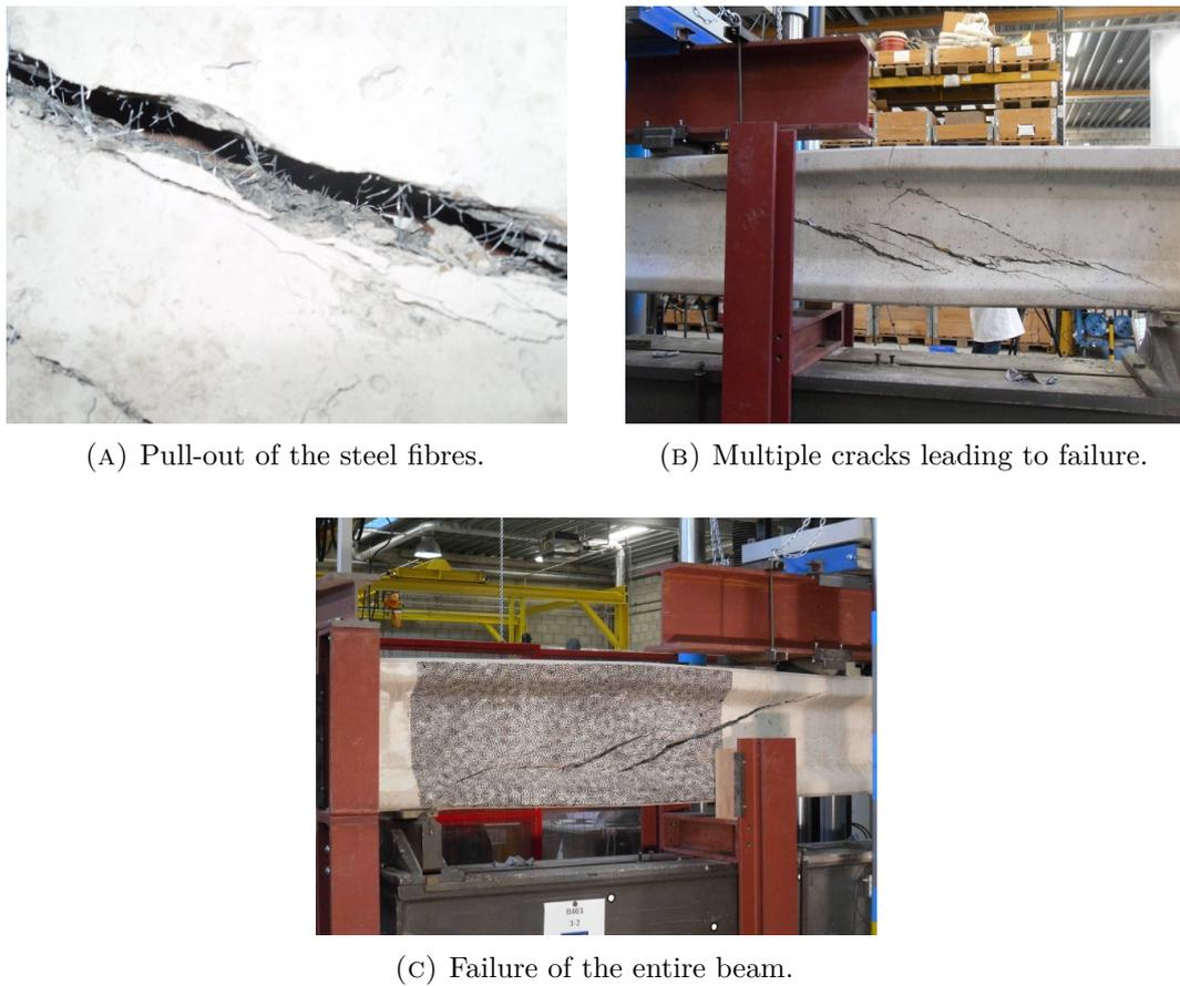
FIGURE 3.43: Different parts of the failure of beam B403.
