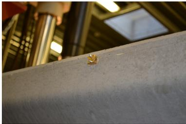
(A) Mechanically anchored optical fibre.
