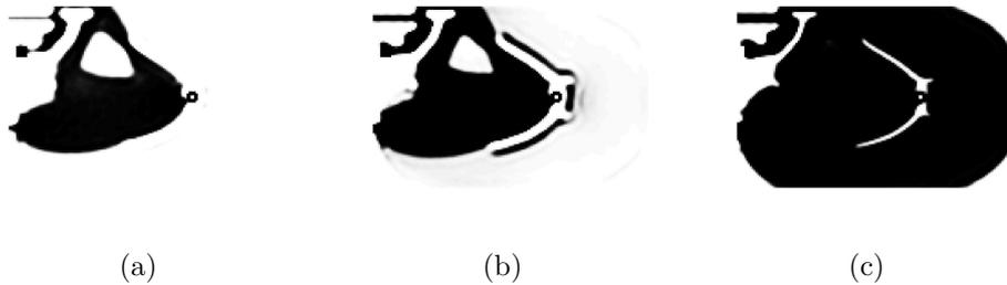
Figure 5.2: (a) Eroded, (b) intermediate and (c) dilated designs of the transducer obtained by the final, most robust topology optimization formulation with the measuring section positioned at one quarter of the height of the transducer.
