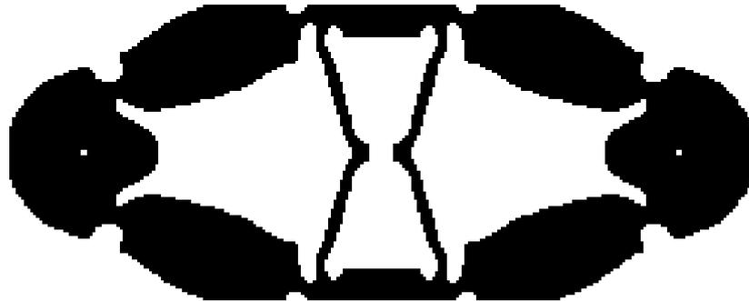
Figure 6.5: Design for the transducer optimized in compression after post-processing.
