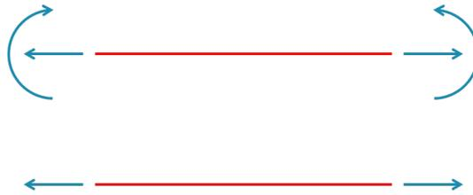
Figure 2.12: Forces occurring in the optical fibre. At the top tension as well as bending, at the bottom only tension.
