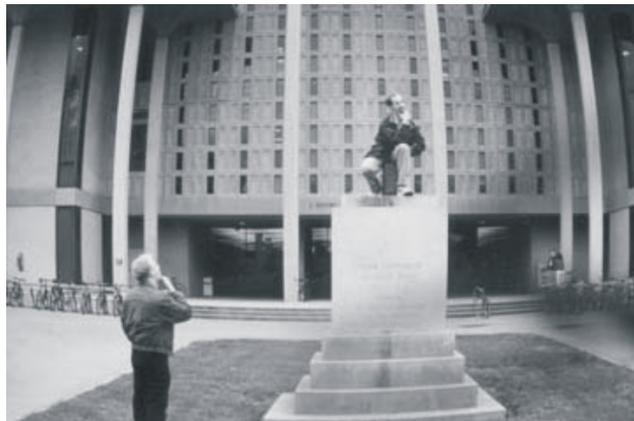
Figure 6.3: An obvious example of radial distortion
