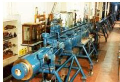
**Figure 3: Mach 6 (right) and the Mach 14 free piston hypersonic wind tunnel (left)**
