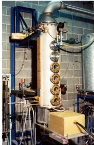
**Figure 2: 15 kW induction-coupled plasma minitorch**
