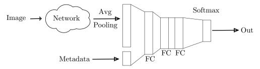
Figure 3.6: Adding metadata to the output fully connected layer while using additional fully connected layers.
