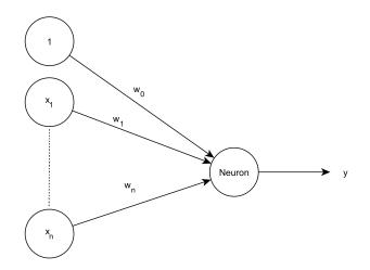
Figure 2.8: A schematic drawing of a neuron is depicted here. Taking all of its inputs  $x_j$  and the corresponding weights  $w_j$ , the neuron calculates an output y.
