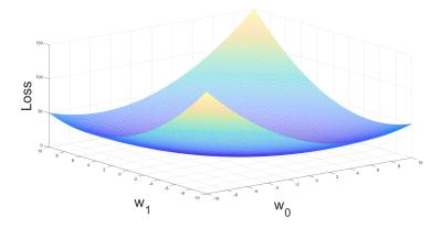
Figure 2.6: Loss function in equation 2.4 with input value  $Z^p = [1,1]$  and required output value  $D^p = 0$ . Notice that there is a minimum where the parameters W will result in the best approximation of the required output. Here  $w_0$  and  $w_1$  respectively are on the x-and y-axes and the loss is on the z-axis.
