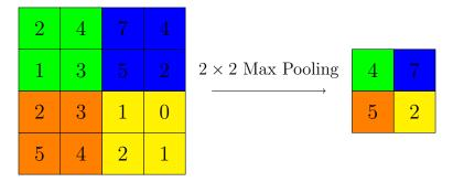
Figure 2.14: Max Pooling according to [22]. The image is divided into  $2 \times 2$  sections, the maximum of each section is taken and finally used to get the values of the downsampled image.
