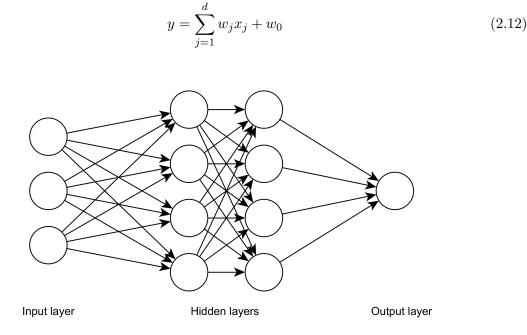
Figure 2.7: Basic representation of a neural network. Each circle is a neuron, while each arrow signifies a connection between two neurons. Note: the *bias unit* is not included in this schematic.
