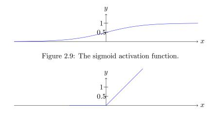
Figure 2.10: The rectified linear unit activation function.
