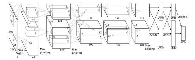
Figure 2.12: AlexNet, as introduced in [42, p. 5].
