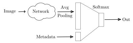
Figure 3.5: Adding metadata to the output fully connected layer without adding any additional fully connected layers. The softmax layer consists of 48 (in the case of species classification) hidden units with the softmax activation function that take the combination of flattened outputs and metadata as input.
