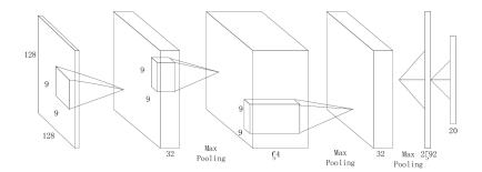
Figure 2.18: The Deep CNN used by Chen et al. to classify cropped camera trap data [3, p. 860].
