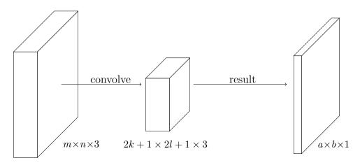
Figure 2.13: The functioning of the convolution layer is demonstrated here.
