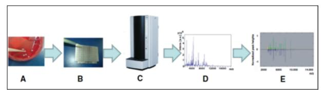
*Figure 3:* A: A single colony is taken from a culture plate. B: The target MALDI-TOF plate is prepared by spreading one colony over each cell of the target plate which is then covered with 1  $\mu$ l of matrix. C: The target plate is inserted in the mass spectrometer. D: A specific sample fingerprint is generated based on time of flight (TOF) information. E: The fingerprint is compared with a reference database for identification (33).
