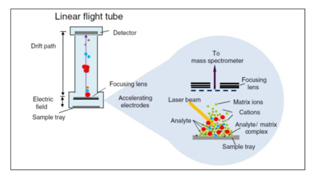
Figure 4: Principle of MALDI-TOF MS (33)
