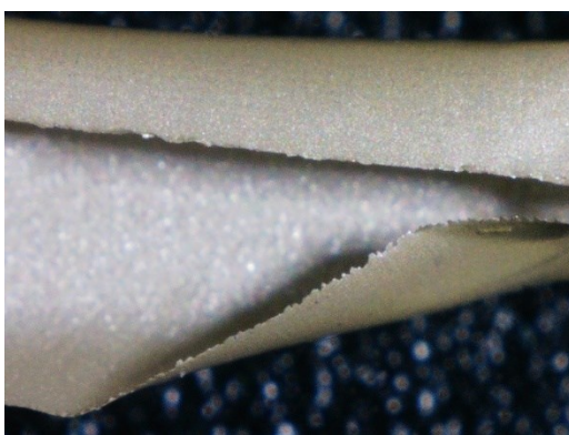
Figure 42: Releasing a sample of ME602 in a sonication bath causes curling of the beam
