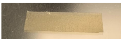
Figure 28: PVA 25 wt% foil sample after treatment at 200 °C. It has been discoloured and its solubility in water is affected
