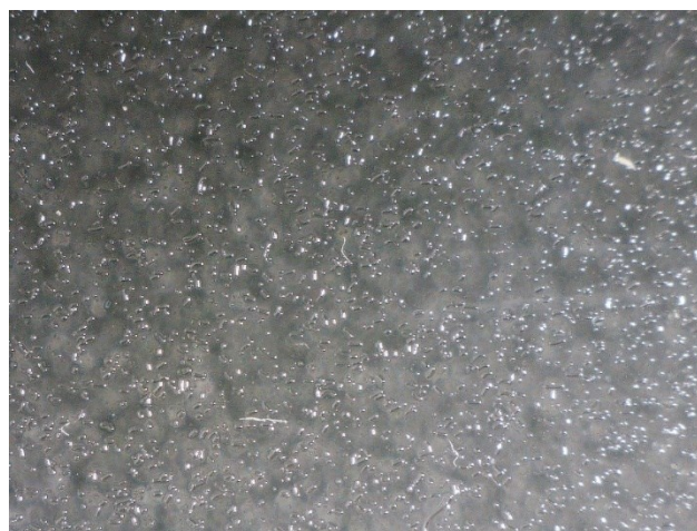
Figure 32: Rough surface of blade coated samples from PVA web 17 wt% ink, unusable as a substrate
